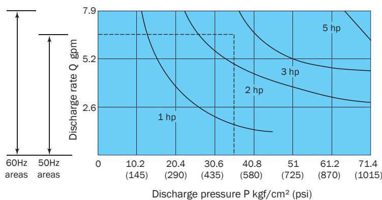
\* Select a uni-pump that has a pressure and flow rate that is within the range of the drive so that the drive will not overload.
